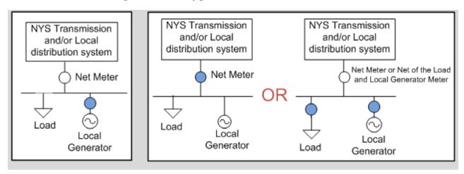
Figure 3: Meter Configurations with On-site Generation/DER
